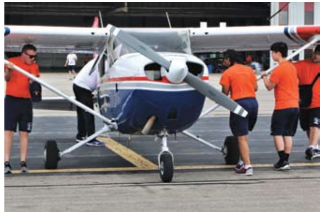
Powered flight students at the Johnson Flight Academy maneuver a CAP Cessna 172 into its parking spot. Note the yellow T-shaped lines painted on the flight line as cadets attempt to line up the plane so they can tie it down. Photo credit: Maj. Greg Hoffeditz, Illinois Wing
