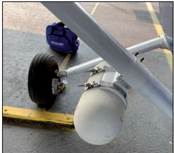
WaldoAir Corp XCAM Ultra50 3D imaging/infrared pod on a CAP G1000 C-182. Photo credit: Lt. Col. Noel Luneau
