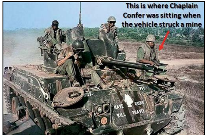
The M42 40 mm Self-Propelled Anti-Aircraft Gun, aka “Duster,” used components from the M41 light tank. Photo credit: Wikipedia
