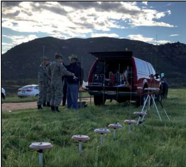
Launch pads set out for rocket mounting. Photo credit: Capt. Mike Hamnquist
