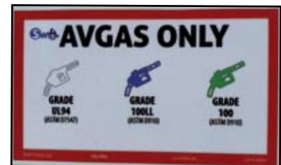
Placard applied to the CAP aircraft based at Reid-Hillview Airport of Santa Clara County indicating that it can now be fueled with UL94. Photo credit: 2nd Lt. Ilya Shabalin
