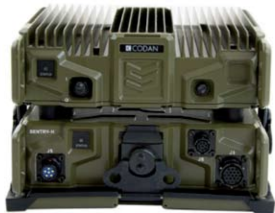
Codan Sentry-H radio and power supply. Photo source: Codan Communications
