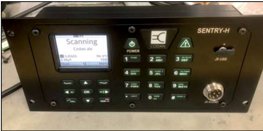
This control head is being built specifically for CAP by Codan. A control head contains the controls for the radio and can be located in a more convenient location when used in a mobile installation. It is connected to the radio's transceiver unit by a cable. Photo source: NVIS Communications
