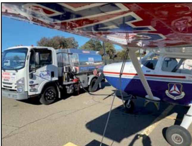
The CAP Cessna 182T being fueled with unleaded fuel, provided by Trade Winds Aviation, at Reid-Hillview Airport of Santa Clara County. Photo credit: 2nd Lt. Ilya Shabalin
