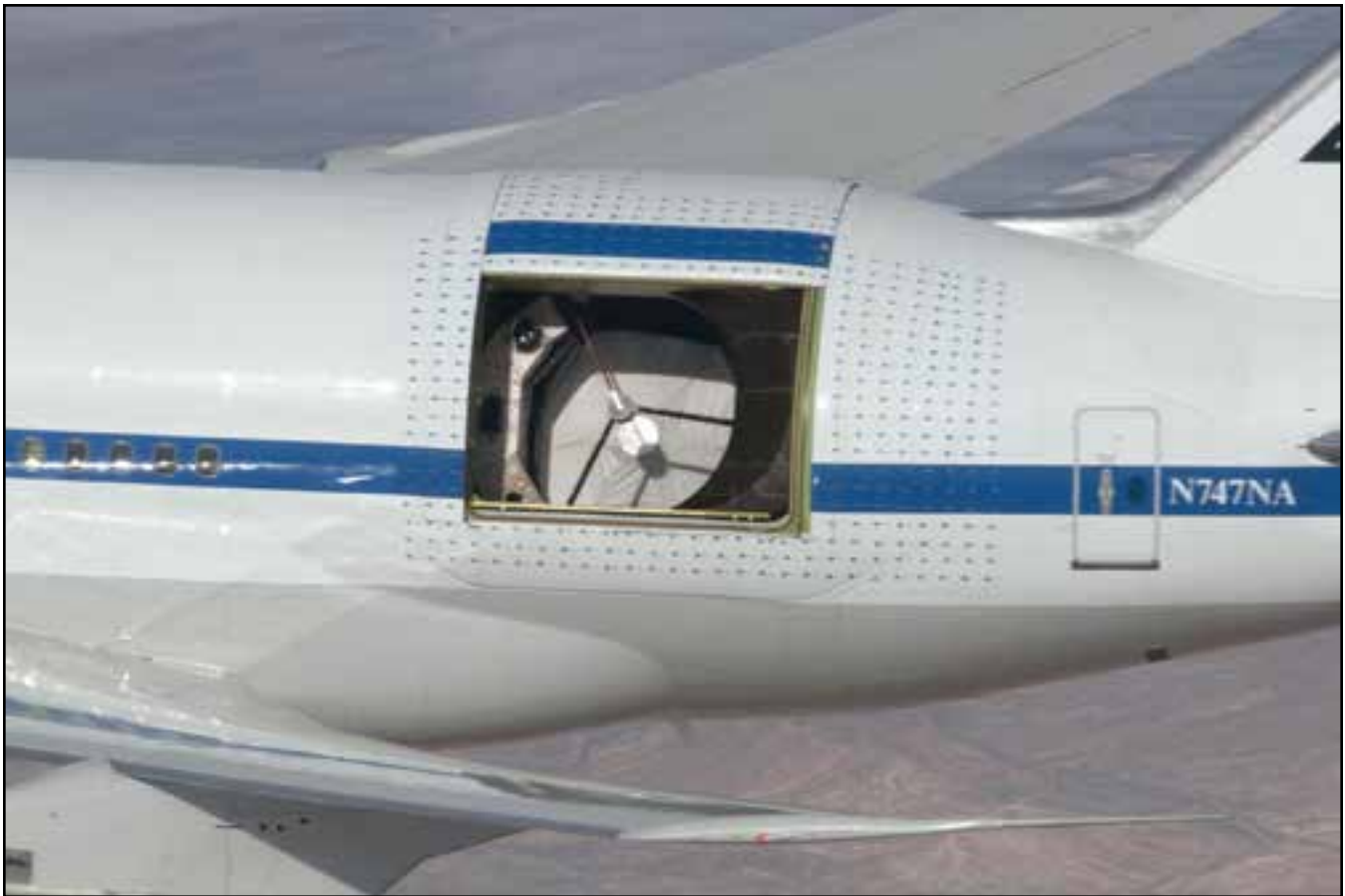
A challenge for the pilot is keeping the large aircraft steady while flying with a 20-ton telescope in a huge cavity in the rear of the plane that is opened to the sky. Photo credit: NASA Armstrong Flight Research Center
