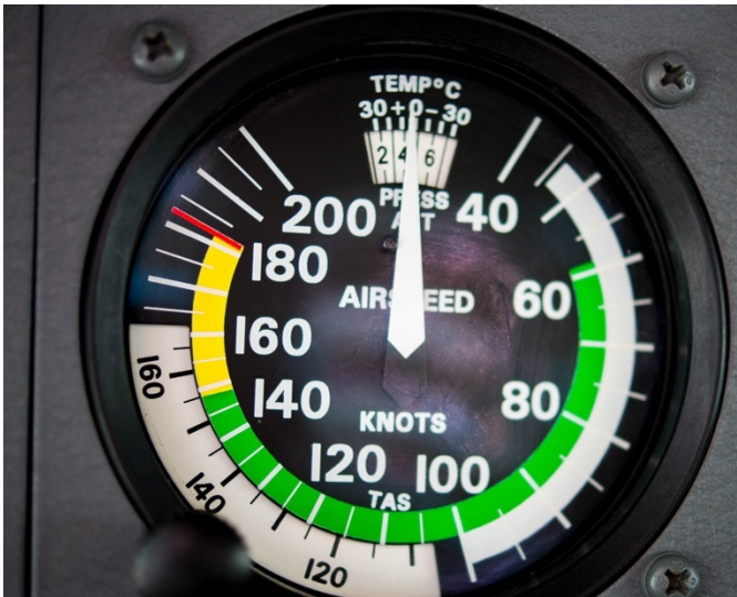
Original Standby Airspeed Note the bottom of the white and green arcs.
