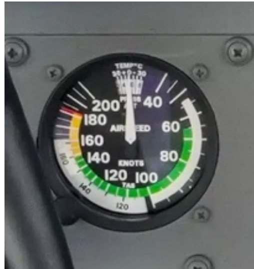
STC Standby Airspeed Note the higher bottom of white and green arcs.
